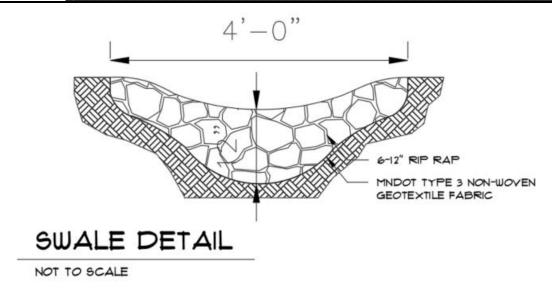
There is no impervious rip rap on the property. All rip rap areas are designed to reduce the velocity, and energy of water, such that the flow will not cause erosion. A permeable geo-textile fabric was used between the rock and existing soil to allow water to pass through.
